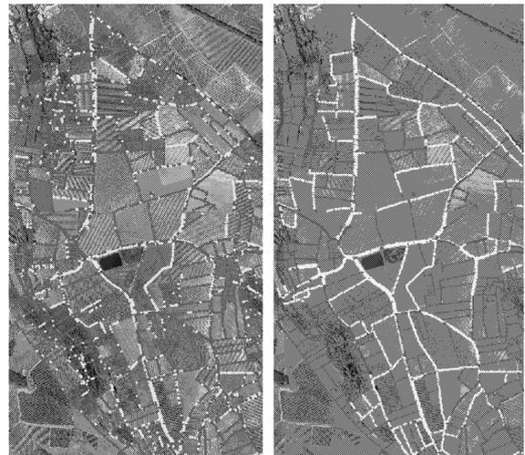
FIG. 6 – Comparison between classification of ditches presence (light grey) on the left and ground truth data on the right for each plot boundary location on the 2km<sup>2</sup> test area
