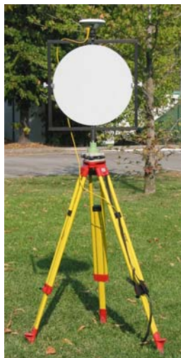
Figure 4: reflective target for TLS applications with GPS antenna mounted
