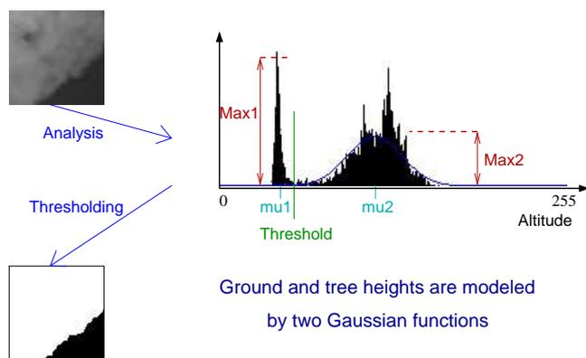
Figure 4: Mixture modelling applied to the histogram
