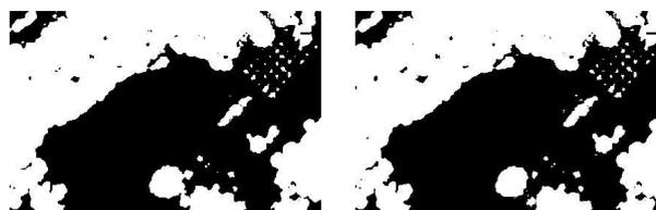
Figure 5: Result of the adaptive thresholding algorithm before correction (left) and after correction (right)
