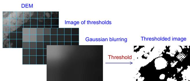
Figure 3: Adaptive thresholding for wooded areas extraction
