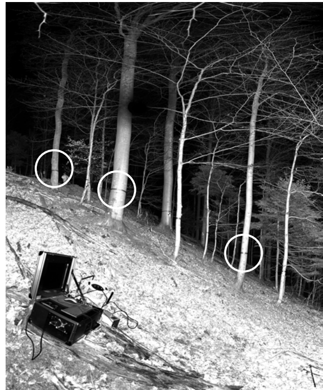
Figure 1. Intensity image of a part of the sample plot. Reflecting tapes mark a height of 1.30 m above ground.
