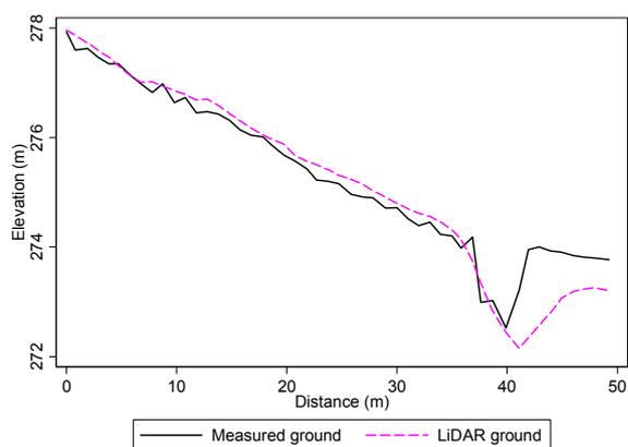
Figure 1. Profiles of measured ground elevation and LiDAR derived ground elevation across the same forest stand
