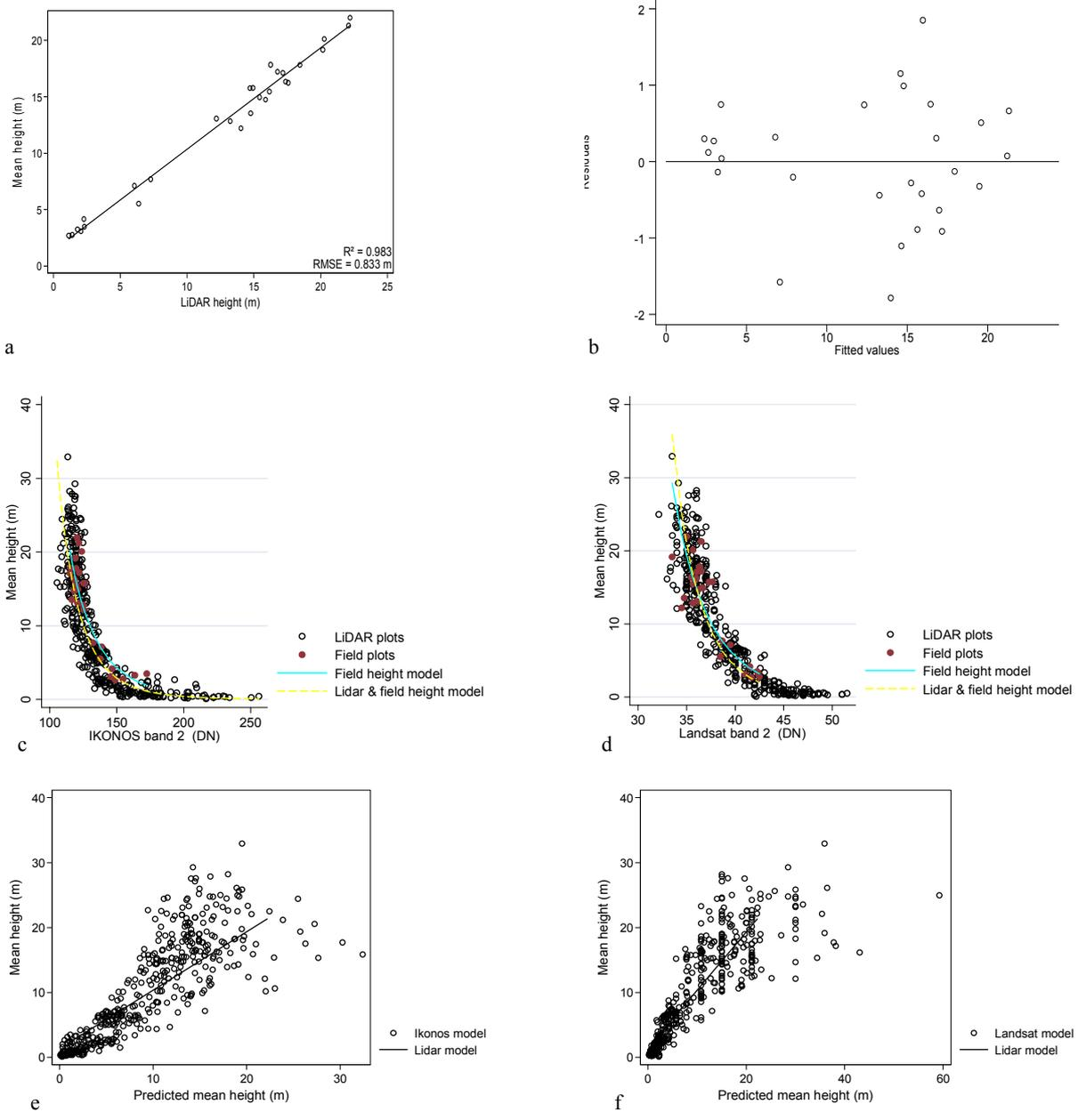
Figure 2. (a) LiDAR height against mean height, (b) LiDAR residual plot, (c) LiDAR height against Landsat Band 2, (d) LiDAR height against IKONOS Band 2, (e) LiDAR height against predicted height IKONOS band 2 (f) LiDAR height against predicted height Landsat Band 2
