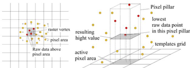
Fig. 1: (Left) Raw data points falling into one pixel area; (Right): Shows the active surface (lowest) and a punch pixel whose height is defined by the lowest raw data point.
