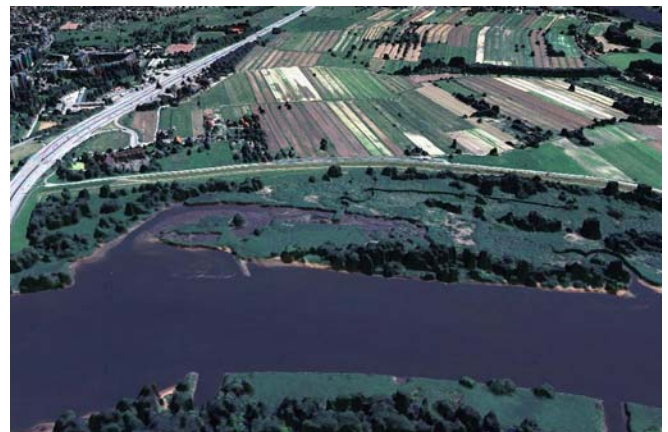
Figure 2: 3D perspective view of a subset of the nature protection area Heuckenlock near Hamburg, Germany. The HRSC-AX image has a ground resolution of 25 cm. The perspective view is a computer generated drape of the RGB image data over the 50 cm resolution digital surface model (DSM) also generated by the HRSC AX.
