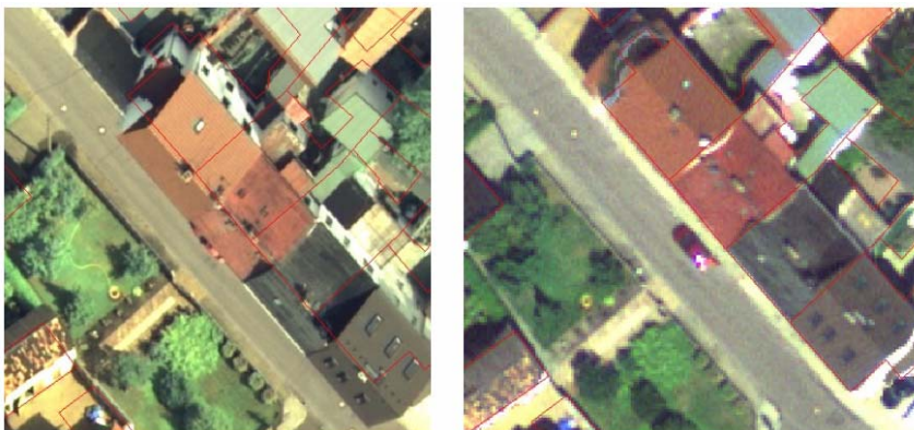
Figure 3 Comparison of the different recording geometries: central perspective DMC (left) and the line scanner ADS (right) with central perspective distortion only in cross-track direction. Digital cadastral data (houses) are overlaid for better clarification.
