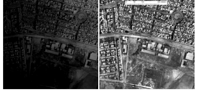
Figure 6: Subset image covered by the smoke plume before (left) and after (right) the radiometric enhancement.
