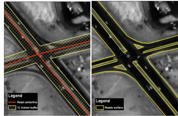
Figure 7: Road center line and derived buffer (left) and digitalized road surfaces (right).
