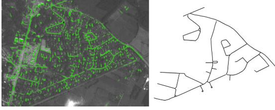
**Figure 1: Left: Ridge detection result in satellite image. Right: Corresponding road vector data**
