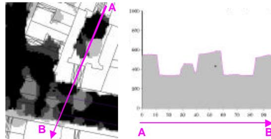
Figure 3. The DSM of the HRSC-AX: useful for detecting complex urban structures.(left: DSM and ALK, right: urban surface profile).
