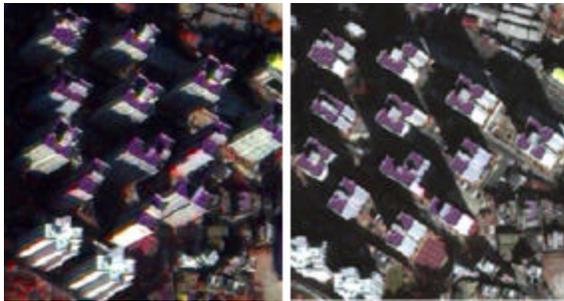
Figure 4. Problem of shadow and inclination of buildings. (left: IKONOS, right: QuickBird).
