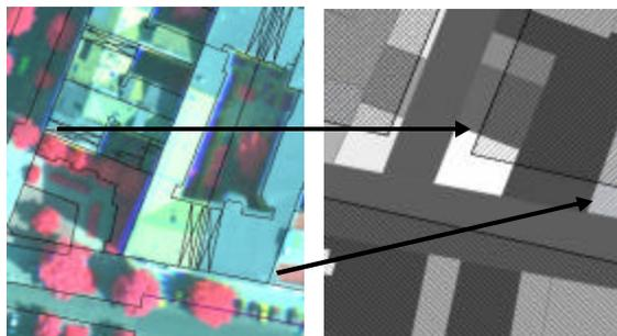
Figure 2. HRSC-AX: Multispectral information with a high geometric accuracy used for visual interpretation to update the old habitat type data (left: multispectral view with automated real estate map; right: new habitat type mapping compared to old data (in hatchings)).
