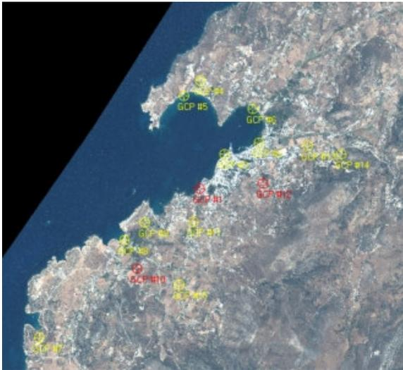
Figure 2 Distribution of the collected GCPs (yellow) and check points (red) during field campaign.
