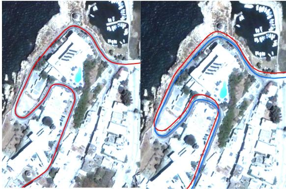
Figure 3 Standard Sharpened True Color type QuickBird image (left) and rectified image using simple linear polynomials with 3D GCPs (right). See overlapped a road segment before (red) and after (blue) the rectification.
