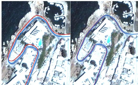
Figure 4 Rectified QuickBird image using the RPC model linearly refined by 3D GCPs (left) and without refinement made (right). In the second case both the rectified (blue) and the non-rectified (red) vectors coincide.
