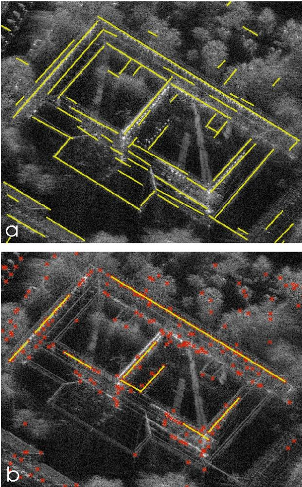
Fig.3 Segmentation results: a) edge and line structures in the two right-angled main directions, b) detected salient point scatterers (red) and groups of those orientated along the main directions.
