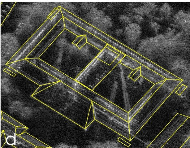
Fig.4 a,b) prismatic and polyhedral 3D city models, c) projection of the building footprints (red) and the roof eave structures into the SAR geometry, d) like c) using the polyhedral 3D city model.
