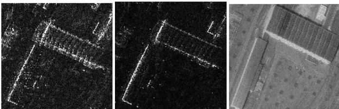
Figure 4: Left and right SAR images used for the correlation
