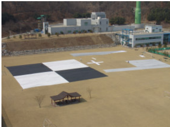
Figure 2. Deployed Tarp target
