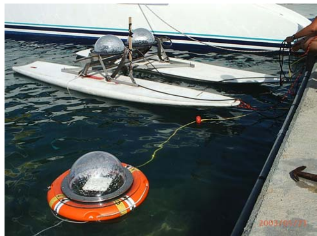
Figure 2. Inter-calibration catamaran/GPS buoy at the Ibiza harbour
