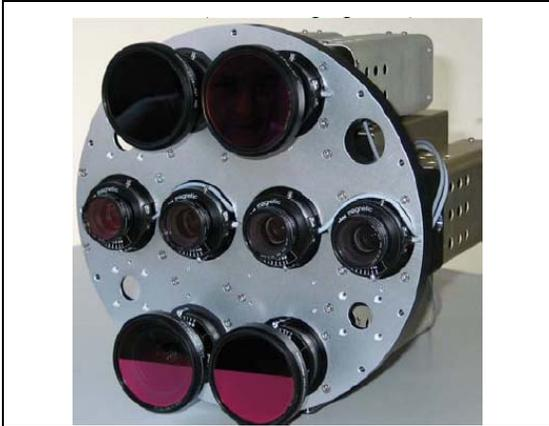
Fig. 7: configuration of UltraCam<sub>D</sub> lenses
