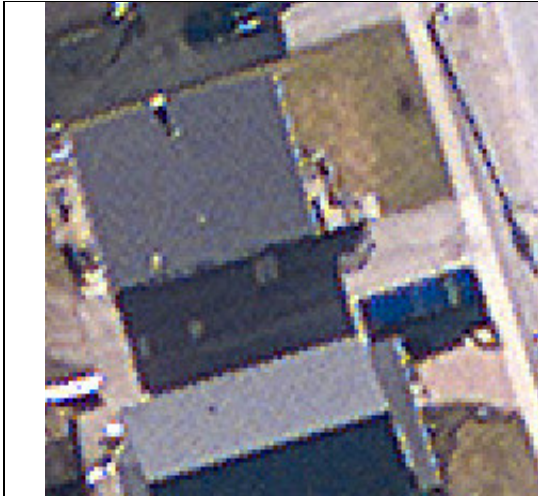
Fig. 2 : samples of color artifacts due to color reconstruction of an image acquire with the Bayer CCD of Applanix DSS322
