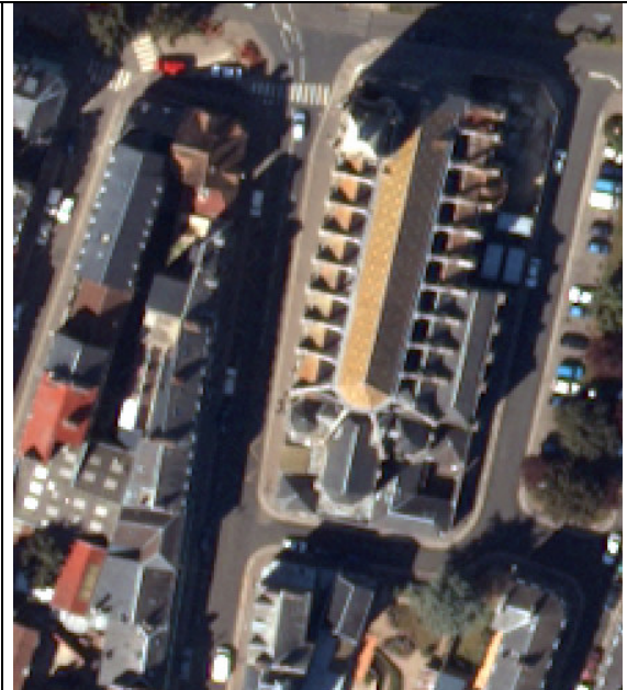
Fig. 1c : the same area resulting of the fusion between GSD 40 cm panchromatic and GSD 68 cm color image
