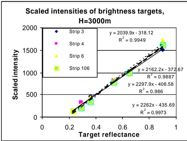
Figure 9. Intensities from strips 3, 4, 6 and 106 scaled to 200 m flying height.
