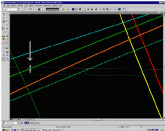
Figure 3. Trajectories over the Sjökkulla test field. The arrow is pointing to the brightness targets. Solid lines describe 3000 m, dashed lines 1000 m and thin dotted lines 200 m flying height trajectories.
