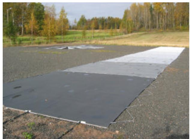
Figure 2. Targets at the Sjökuilla photogrammetric test field in Kirkkonummi arranged for a digital aerial camera test. (Photo 4 Oct. 2004 by H. Kaartinen).
