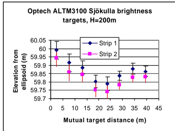
Figure 4. Averages and standard deviations of elevations of the targets.
