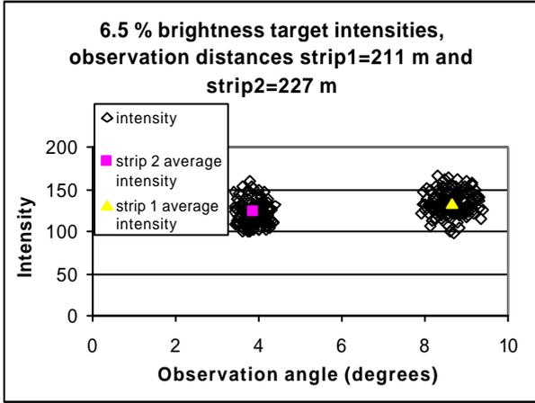
Figure 5. The relation between the intensity and observation angle is distorted by the range difference of the two strips.
