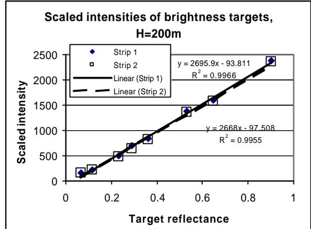
Figure 7. Intensities from strips 1 and 2 scaled to 200 m flying height.
