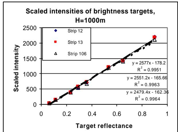
Figure 8. Intensities from strips 12, 13 and 106 scaled to 200 m flying height.
