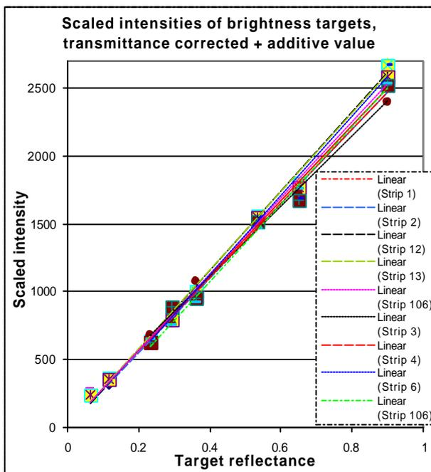
Figure 12. Intensity values corrected for atmospheric transmittance and additive values from regression lines.
