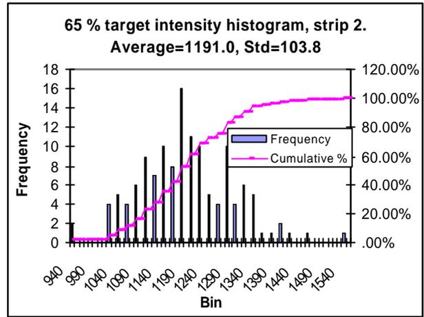
Figure 10. Histogram of beam intensity with 65 % target reflectance. Flying height 200m.
