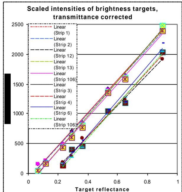
Figure 11. Intensity values corrected for atmospheric transmittance.
