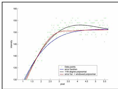
Figure 5. Different ESF models at higher corner
