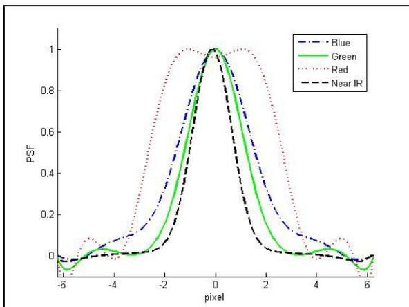
Figure 6. PSF curves for multispectral imager channels
