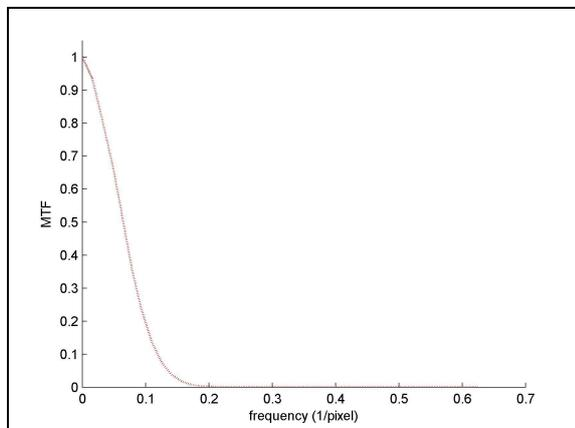
Figure 13. MTF of panchromatic channel
