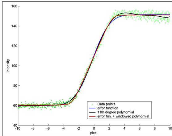
Figure 4. ESF curves for red channel
