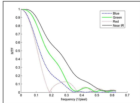
Figure 7. MTF curves for multispectral imager channels
