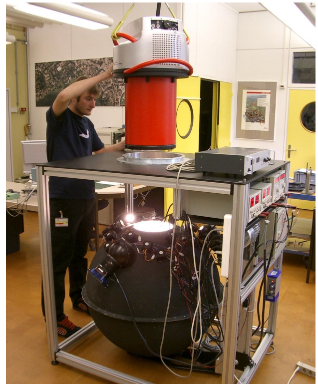
Figure 3. Spectral calibration and MTF measurement unit at Leica Geosystems
