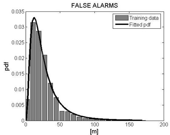
Figure 5. A lognormal distribution is fitted to a histogram of the attribute length (FALSE\_ALARMS).
