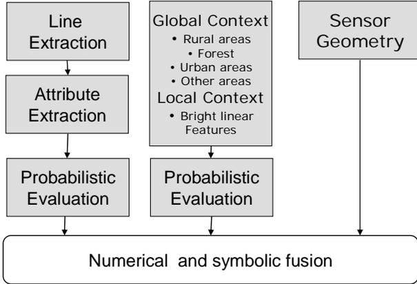
Figure 2. Fusion module and its input data
