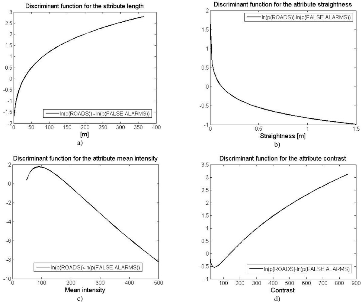
Figure 6 a-d. Discriminant function for the attributes a) Length, b) Straightness, c) Inner intensity and d) Contrast.
