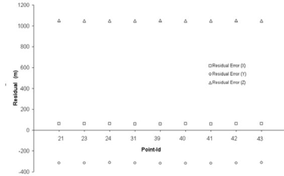
Figure 2. The error plot in X,Y,Z in no-GCP scenario
