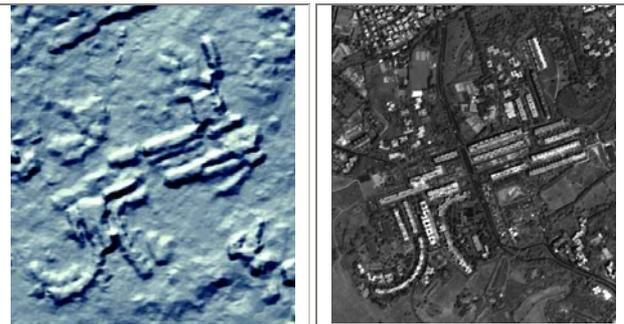
Figure 6. 5m-cell CartoDEM and corresponding AFT orthoimage
