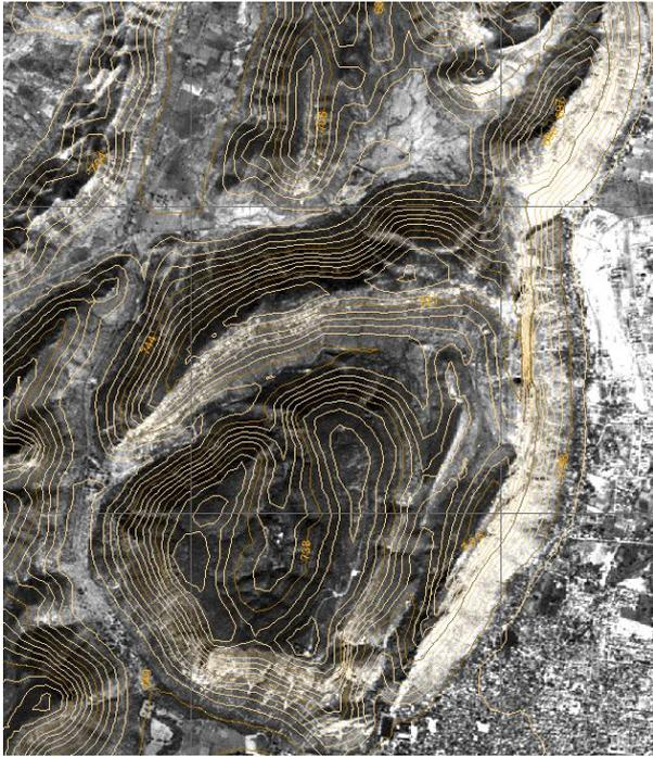
Figure 7. Detailed view of orthoimage with 20 m contours.
