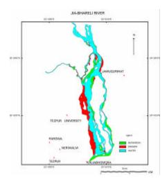
Also, the river has shown a distinct channel shifting from east to west which is shown in the following fig. (2).
