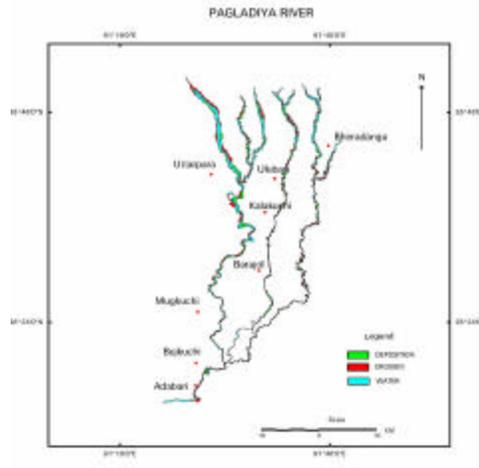
**Fig: 6 erosion/deposition in Pagladiya**
