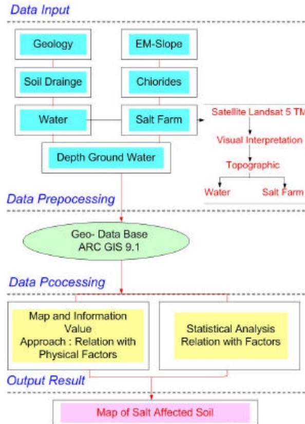
Figure 2. Flow hart of creating and integrating GIS coverage with data map
