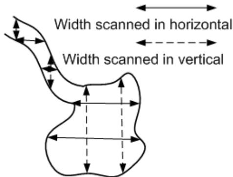
Figure 4: Elimination of non-channel segment part using scanned widths in horizontal and vertical.
