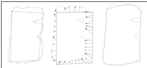
Fig. 8: Poor results alignment results due to insufficient vertex distribution.
