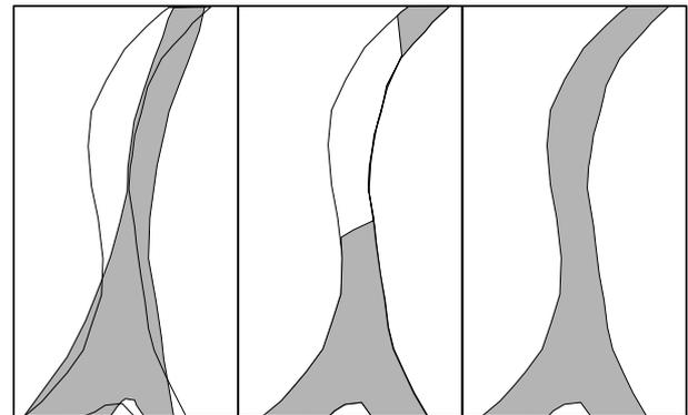
Fig. 1: Left – Aligning a river from a reference (dark border) and a candidate data set (filled), Middle – candidate object misaligned, Right – candidate object aligned with estimating segment orientation
