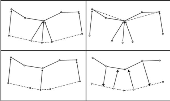
Fig. 5a-d: (First row, left) Relation based on distance evaluation, (right) resulting in an invalid geometry and unrelated vertices. (Second row, left) Selection of shortest neighbor, (right) allocation of new targets.
