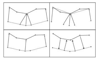
Fig. 5a-d: (First row, left) Relation based on distance evaluation, (right) resulting in an invalid geometry and unrelated vertices. (Second row, left) Selection of shortest neighbor, (right) allocation of new targets.
