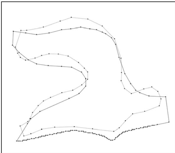
Fig. 4a: Object with very irregular distribution of vertices (dark line), and target object (dotted line).
