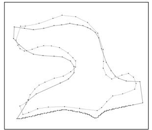
4a: Object with very irregular distribution of Fig. vertices (dark line), and target object (dotted line).
