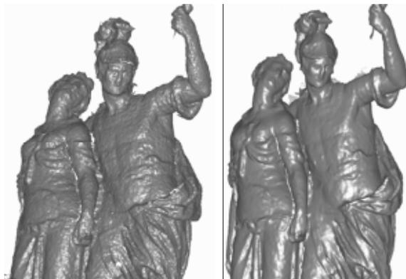
Figure 10: Example of 3D point cloud. Left: unfiltered point data. Right: filtered data using the robust Fast Minimum Covariance Determinant (FMCD) method
