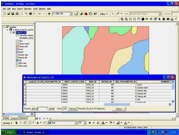
Fig. 6a Seabed sediment distribution map generated in desktop ARC GIS fetching attribute data from Oracle tables
