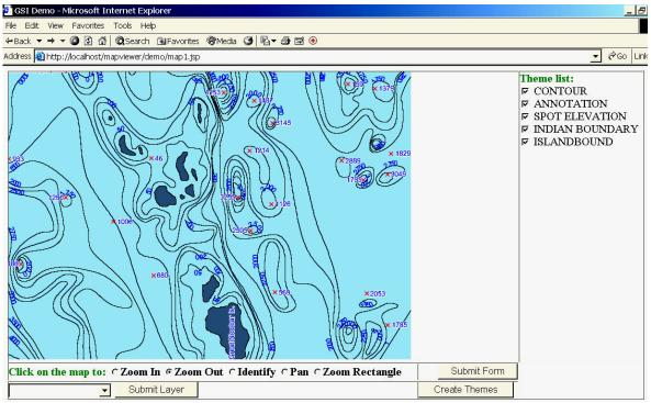
Fig. 6b. Display of bathymetric map through Map Viewer in the browser-based environment fetching data from Oracle Spatial tables
