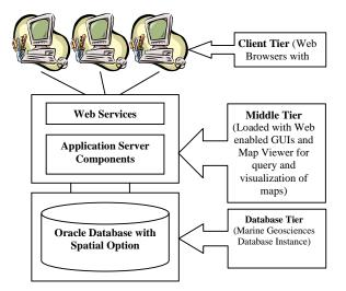
Fig. 3 : Three-Tier Database Architecture Model adopted for Marine Geosciences database
