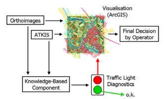
Figure 1: Workflow implemented in WiPKA
