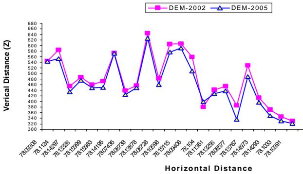
Figure 4. Minimum and Maximum height of control points in DEM-2002 and DEM-2005
