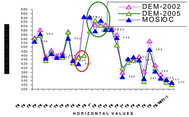
Figure 6. Minimum and Maximum height of control points between DEM-2002, DEM-2005 and Mosaic.
