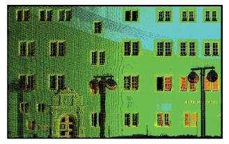
Figure 7: Laser point cloud to be used for the geometric refinement of the corresponding building façade.
