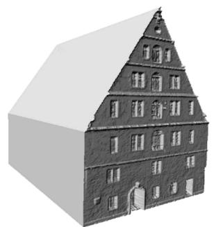
Figure 6: Refined visualisation of building façade using displacement mapping.
