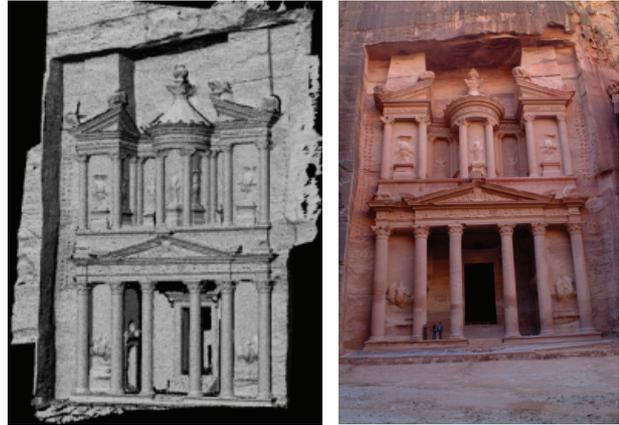
Figure 1: Meshed 3D model from terrestrial laser scanning (left) and texture image from independent camera station (right).
