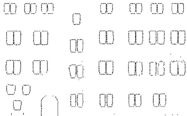
Figure 8: Detected edge points at horizontal and vertical window structures.
