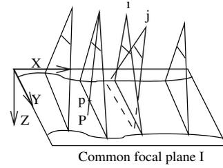
Figure 3: Reprojection of all pixels onto a common focal plane.
