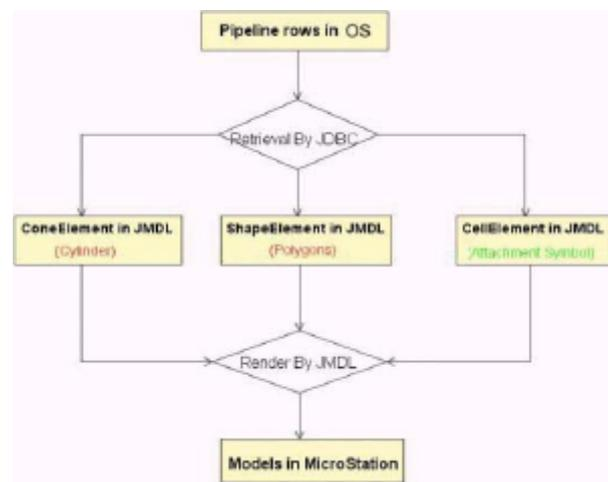
Figure 2: On-the-fly creation of 3D shapes for visualisation. Using this approach, three programs for visualization of 3D pipelines are developed (Figure 2): 1) circular pipeline, 2) rectangular pipeline, and 3) 3D symbols. The following text presents the algorithms.
