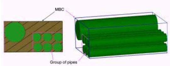
Figure 4: Rectangular pipelines as MBC of cable groups
