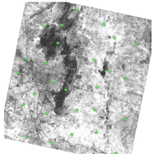
Figure:3 GCP Distribution: Jaipur
