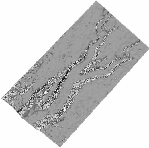
Figure 5: Hillshade view on Model No. 1 produced manually on an analytical plotter WILD S9
