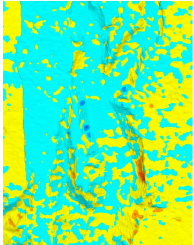
Figure 6: Differences between manual measurements and SAT-PP results for Model No. 1. (Large differences are dark, small differences light)
