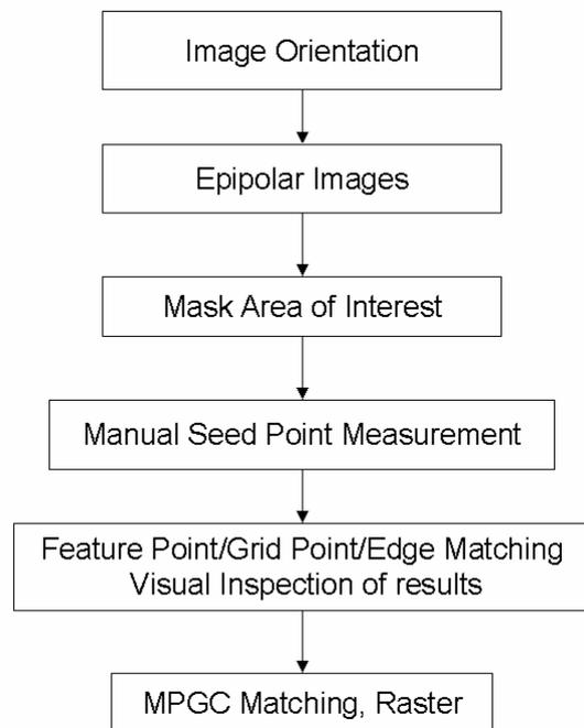
Figure 3: Workflow for DSM generation in SAT-PP
