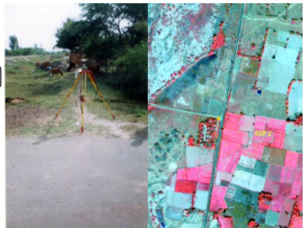
Figure3: Field Photograph and Corresponding Image Position
