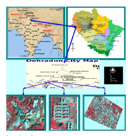
Remote Sensing Data *IKONOS 1m Panchromatic* Spectral range: 0.45 - 0.9 micrometers. Data: 11 bits per pixel (2048 grey tones) *IKONOS 4m Multispectral* Band 1: 0.45 - 0.53 (Blue), Band 2: 0.52 - 0.61 (Green),Band 3: 0.64 - 0.72 (Red),Band 4: 0.77 - 0.88 (Near Infrared
