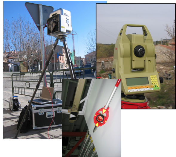
Figure 2. 3D laser scanner Trimble GS200, Leica TPS 1000 total station and the Leica mini-prism
