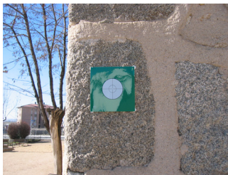
Figure 5. Target used as tie point for the point cloud merging, as well as control point
