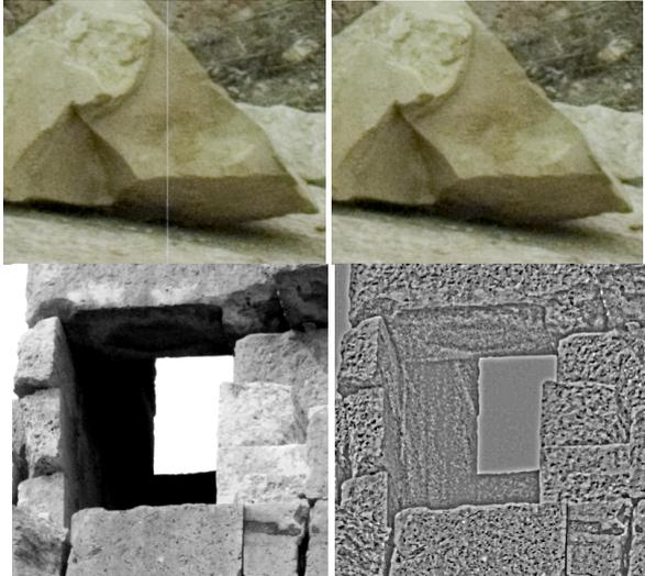
Figure 4: Results of the column pixel defect correction (top middle) and image enhancement, especially in dark regions, by means of Wallis filter (bottom, before and after Wallis).
