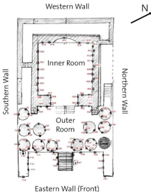
Figure 2: An overall view of the Artemis temple in Jerash, with some of the control points in the inner and outer room and front part.
