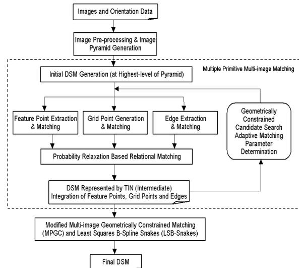
Figure 5: Workflow of the automated DSM generation approach. The approach consists of three mutually connected components: the image
