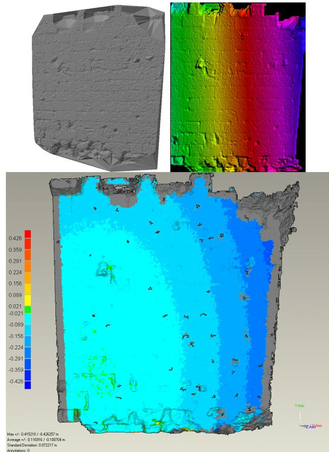
Figure 7: DSM generated using LPS and our in-house matcher (above, left and right) and 3D comparison between the two results (below).
