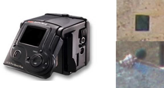
Figure 3: The used Kodak DCS Pro Back Plus camera (left) and the signalized tape and tennis ball control points (right).
