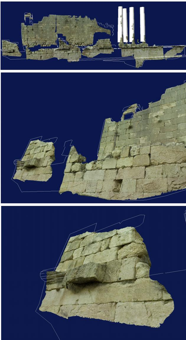
Figure 6: Some views of the textured 3D model of the south side of the Artemis temple. Most part of the surfaces are automatically reconstructed with a multi-photo surface matcher, except the columns and some object edges which are manually measured with PhotoModeler.
