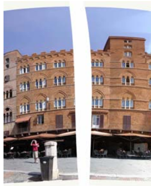
Figure 13 - The correction with georeferencing function of ArcGis. The two tails of the image are deformed and they are no more coinciding as they should be
