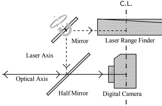
Figure 2. Configuration of the IBIM system
