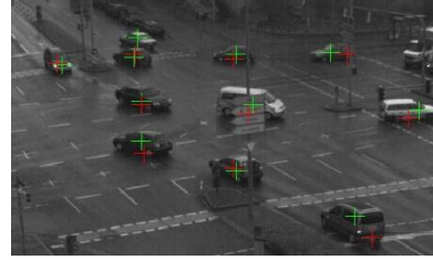
Figure 15: Influence of shadow inclusion on shape centroid: green — reference, red — output of image processing 1
