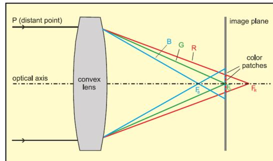
Figure 5: Longitudinal aberration
