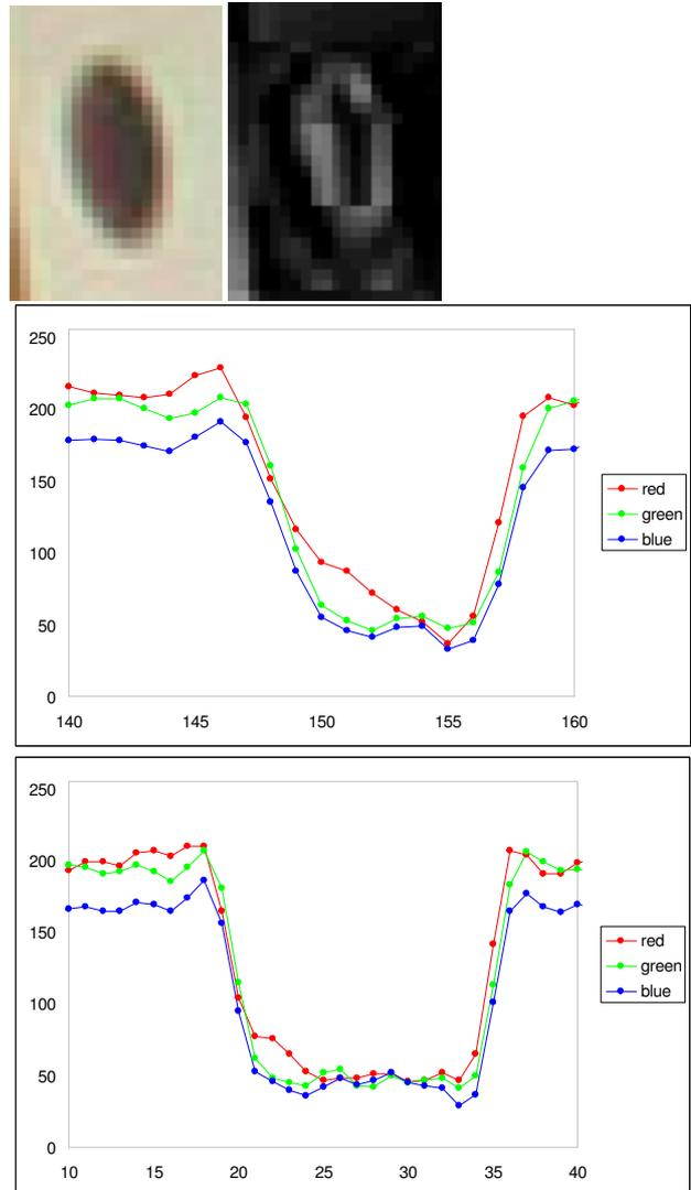
Figure 11: Sample target (Figure 7), top-left: after manual correction of chromatic aberration, top-right: red minus green band (stretched), middle and bottom: RGB profile in column direction of a small and a large target.
