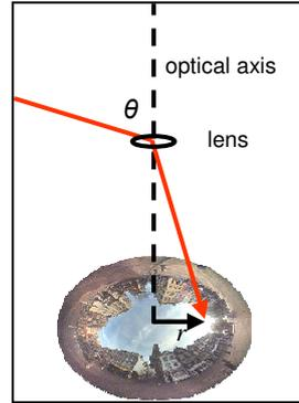
Figure 3: Fisheye projection (schematic).
