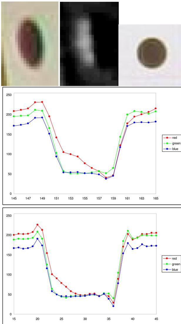
Figure 7: Sample target (small) located close to the right image border (Figure 4), top-left: original, top-middle: red minus green band (stretched), top-right: target in image centre, middle and bottom: RGB profile in column direction of a small and a large target.
