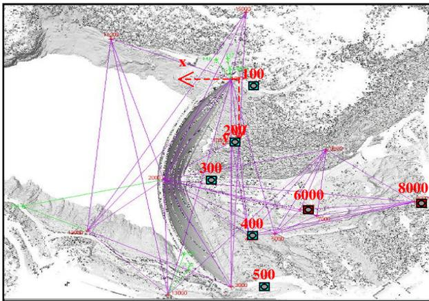
Fig. 3.- Layout of the geodetic network reporting laser scanner stand-points.
