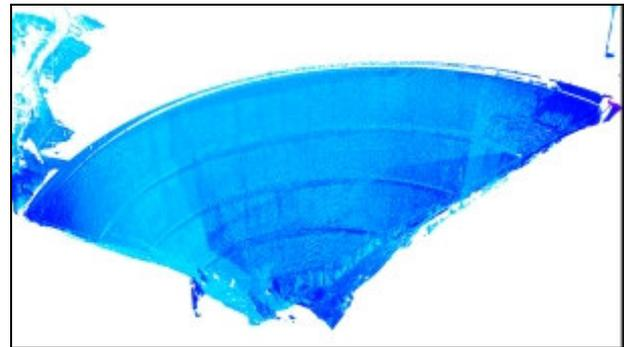
Fig. 4.- Point-cloud resulting from data fusion of all scans capturing dam downstream face acquired by Leica HDS 3000.
