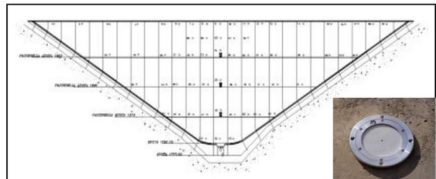
Fig. 2.- Positions of targets to be used as independent control points on the dam's front; in the window on the left, an image of a retro-reflecting target used for Riegl LMS-Z420i laser scanner.
