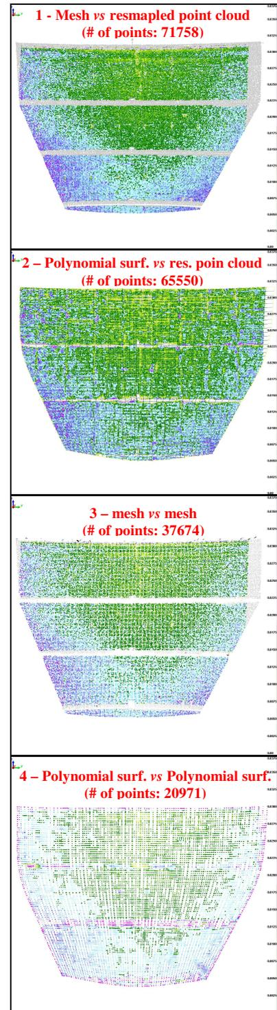
Fig. 5.- Maps of deformations evaluated by comparing different kinds of surfaces derived from scan acquired from station 8000 in Oct 2005 and May 2006.
