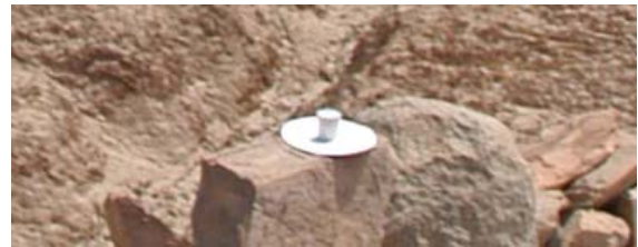
Figure 3. A signalized control point for both laser and UAV data orientation.
