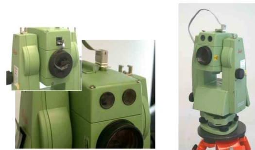
Figure 6. Combination of imaging system and tacheometer developed by Scherer (2006).
