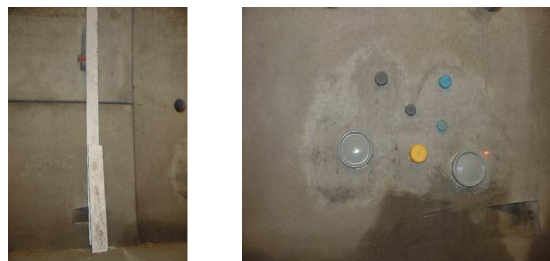
Figure 4. Artificial deformations placed against the tunnel wall.
