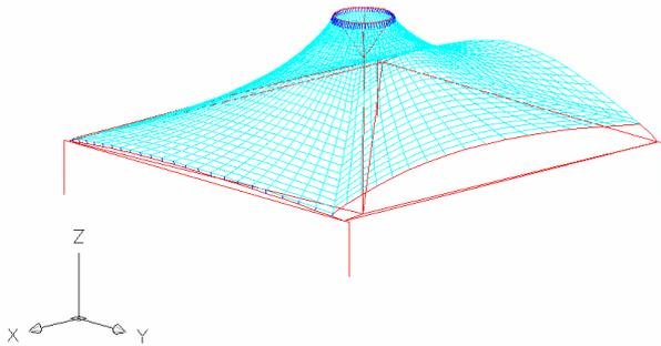
Figure 2. Mathematical model of the membrane roof structure.
