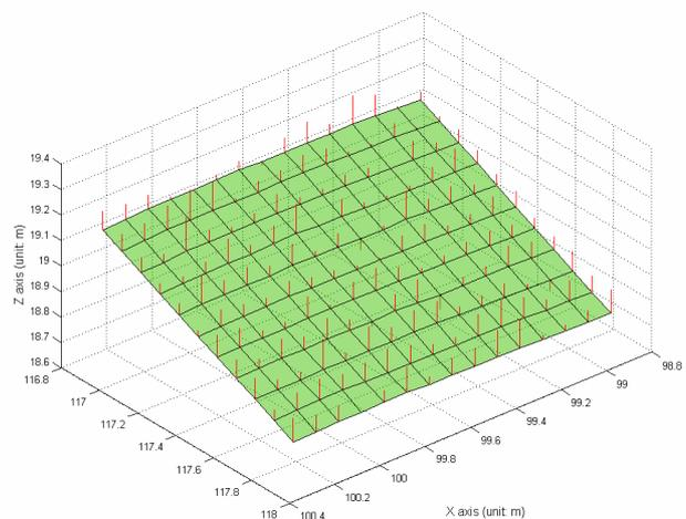
Figure 10. Close-up view of the displacement of the observed surface. The base is the surface model of the 1<sup>st</sup> epoch, the vectors (which is ten times magnified) represent the differences to the 2<sup>nd</sup> epoch.
