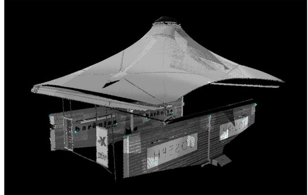
Figure 3. Laser scanned model of the membrane structure.
