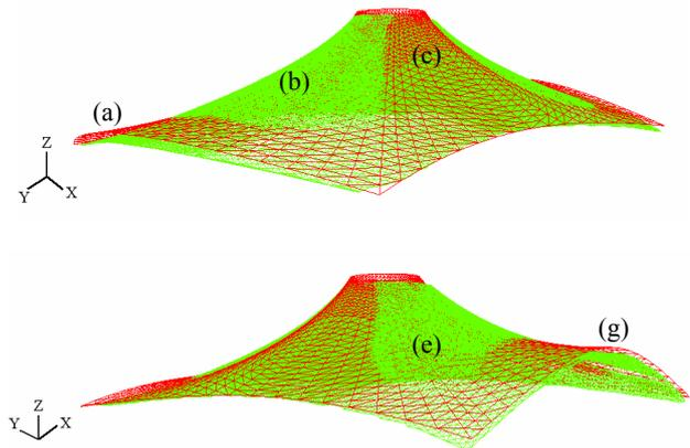
Figure 5. Resultant meshed models after surface matching (green mesh: laser scanned model; red mesh: transformed mathematical model).
