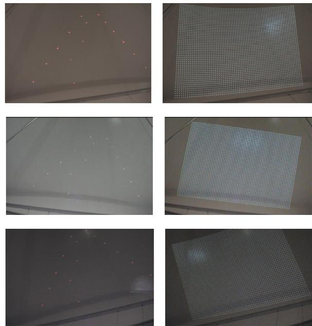
Figure 7. Images of control points (left) and example frames of projected targets (right).
