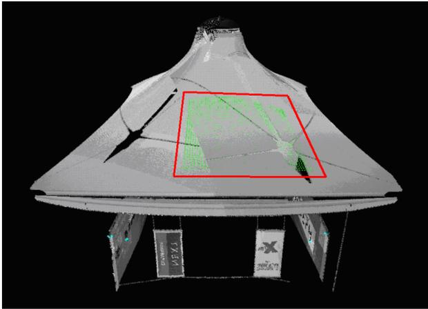
Figure 11. Laser scanned (monochrome) and videogrammetric (green points outlined by red line) models.
