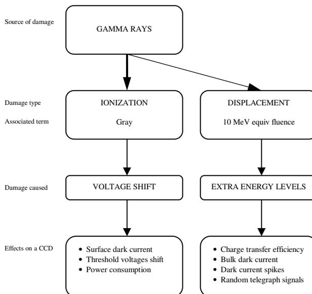
Figure 1. The radiation damage tree for CCDs. Illustration from (Bassler, 2004)
