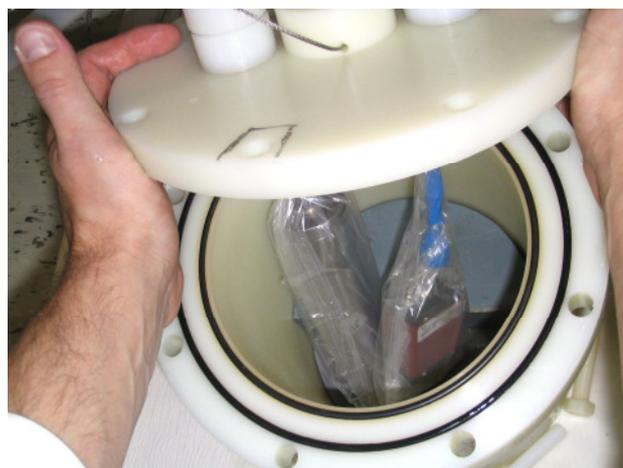
Figure 3. Polyethylene container which carries camera and radiation sensor.
